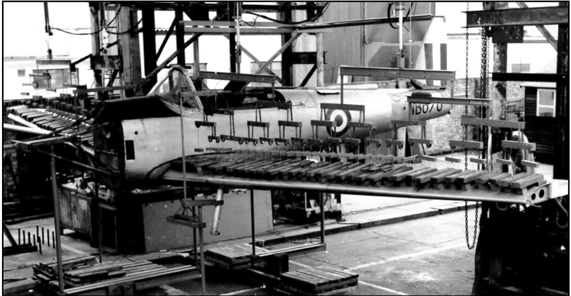
**FIG. 3. DHC-1 CHIPMUNK T MK 10 - FULL-SCALE FATIGUE TEST**
